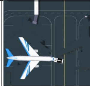
Frame 7: Pilot receives control immediately after pushback has been completed.
