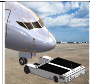
Frame 4: Ground crew personnel align the tug with the aircraft nose wheel.
