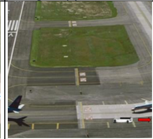
Frame 12: Aircraft engines start, pilot continues to takeoff and the tug returns autonomously or via Tug Operations Center. [21]
