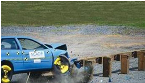
Figure 1. Full-Scale Crash Test. (Source: FHWA.)
