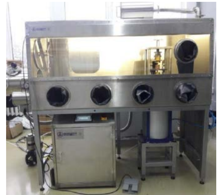
RF: High-Voltage Compaction Method for production of Fuel Pellet (Lab-Scale)
