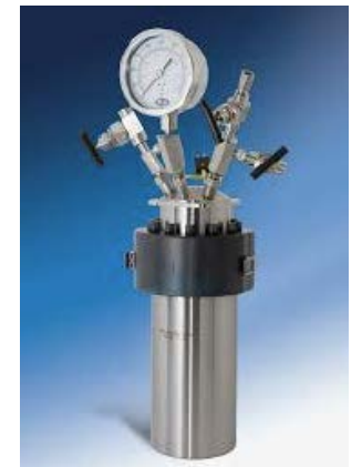
Euratom: MA-bearing transmutation oxide-based fuel synthesis device using Hydrothermal Decomposition
