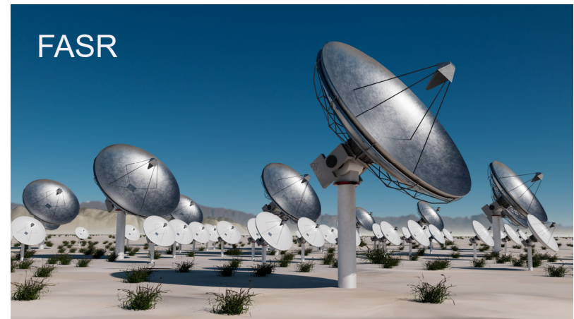
FASR MSRI-2: Frequency Agile Solar Radiotelescope – A 3D radio “camera,” observes the Sun’s atmosphere as a coupled system
