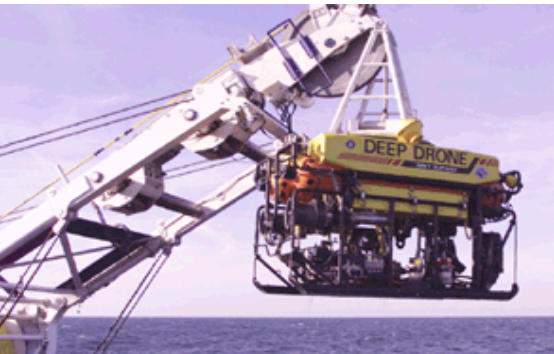
Deep Drone ROV Depth - 8,000 ft
