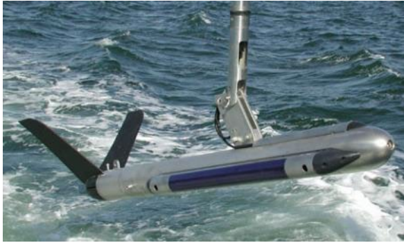
Shallow Water Intermediate Search System (SWISS) Depth - 7,000 ft
