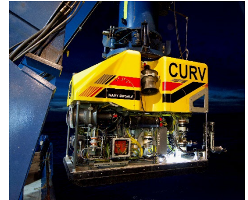
Cable-Controlled Underwater Recovery Vehicle (CURV) 21 ROV Depth - 20,000 ft
