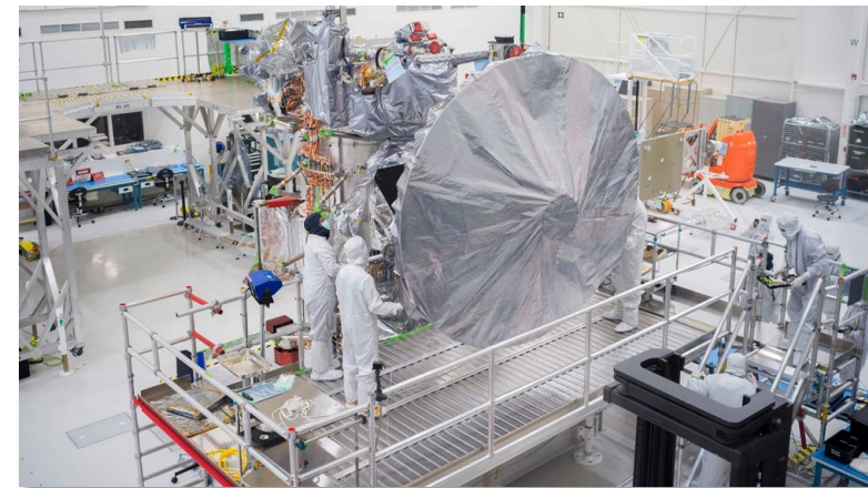
Installation of 10-ft high-gain antenna
