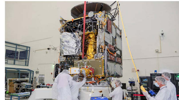
Engineers at NASA's Jet Propulsion Laboratory work to integrate Hall thrusters into the agency's Psyche spacecraft in July 2021. One of the thrusters is visible on the side of the spacecraft underneath a red protective cover. Credits: NASA/JPL-Caltech
