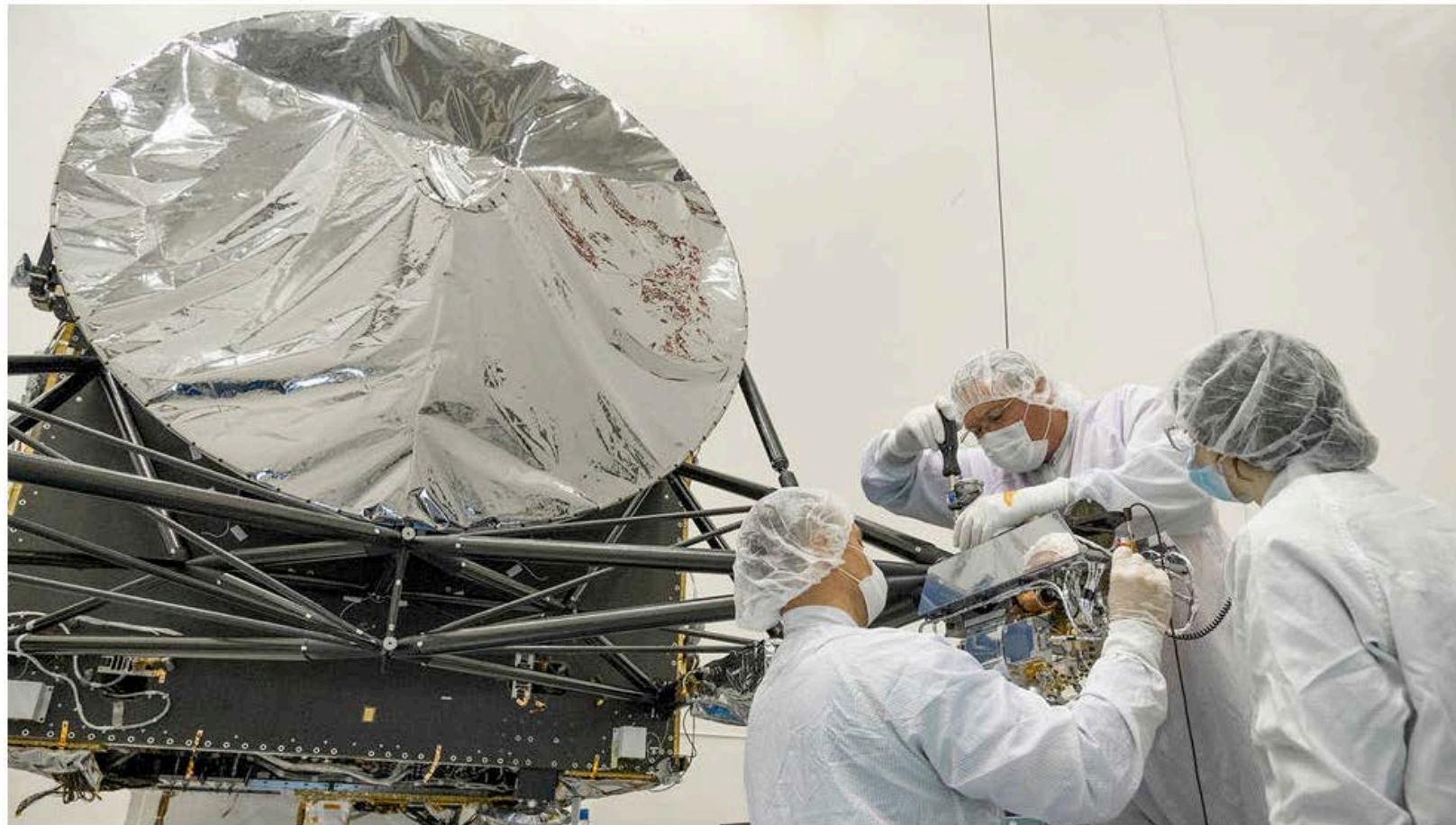
At NASA's Jet Propulsion Laboratory, engineers integrate a gamma ray and neutron spectrometer into the agency's Psyche spacecraft. The instrument will help determine the elements that make up its target, an asteroid also named Psyche.
