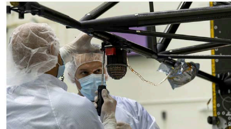
Engineers at NASA's Jet Propulsion Laboratory in Southern California integrate the magnetometer instrument into the agency's Psyche spacecraft on June 28, 2021. The instrument will help determine if the Psyche asteroid is part of a planetesimal, the building block of an early planet. Credits: NASA/JPL-Caltech
