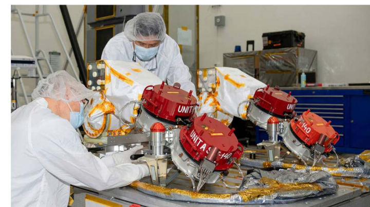
At NASA's Jet Propulsion Laboratory, engineers prepare to integrate four Hall thrusters (beneath the red protective covers) onto the agency's Psyche spacecraft. The thrusters will propel Psyche to its target in the main asteroid belt. Credits: NASA/JPL-Caltech
